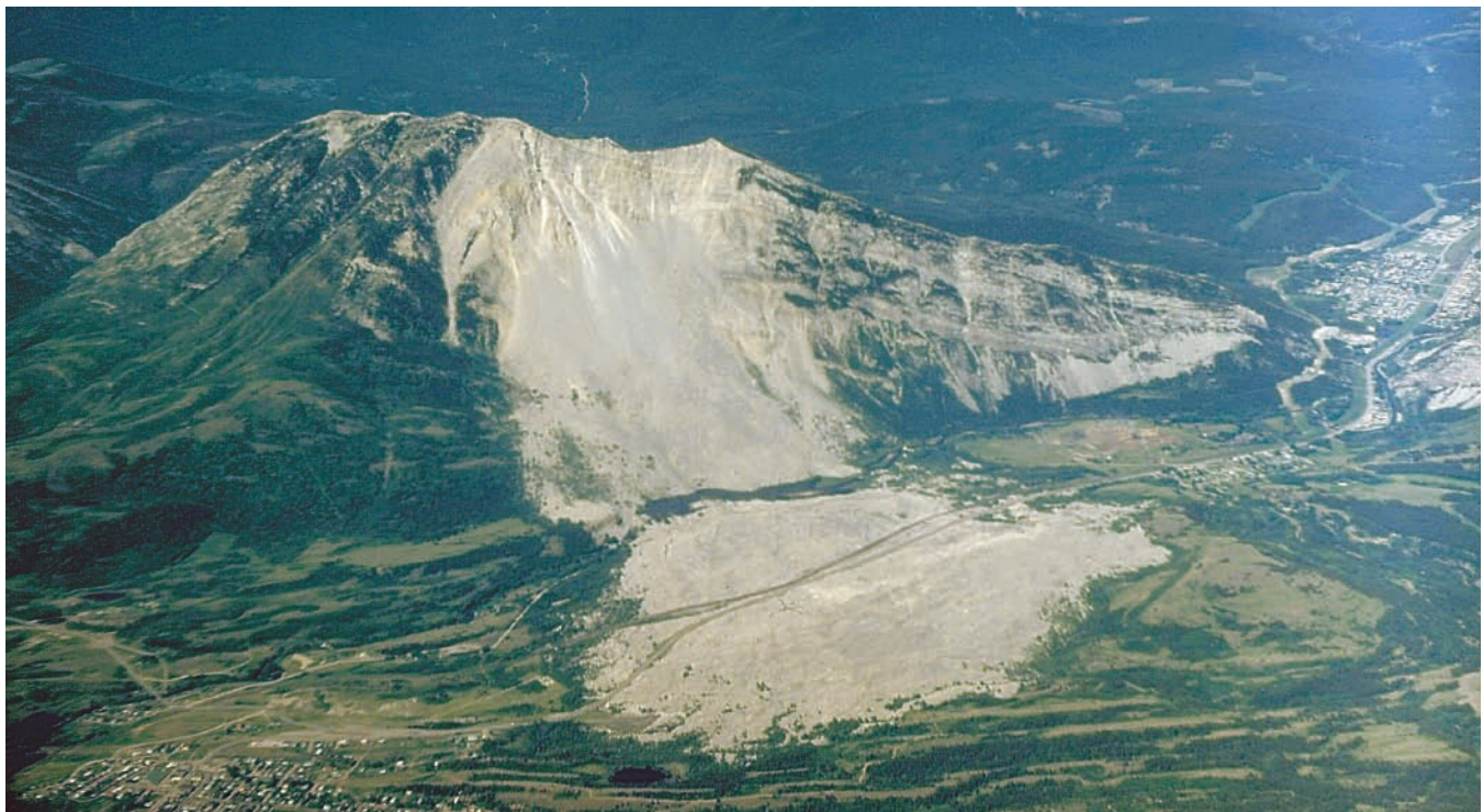
FIGURE 11.11 The Frank rockfall, Alberta, Canada, involved a huge mass of rock that broke away from the mountain face, completely burying the mining town of Frank, Alberta. Among the factors that contributed to this slope failure were the steepness of the mountain front, the dip of the bedding planes parallel to the mountain face, and underlying weak shale and coal beds. Mining activity may have triggered the movement. (Courtesy of P. Nixon)
